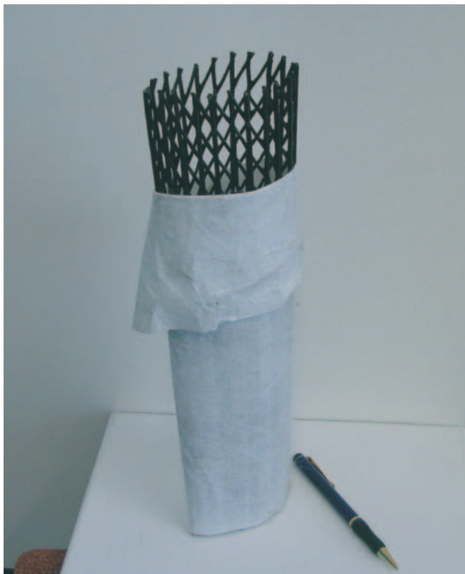
Fig. 3. View of electrokinetic geosynthetic (EKG) used in the tests.
