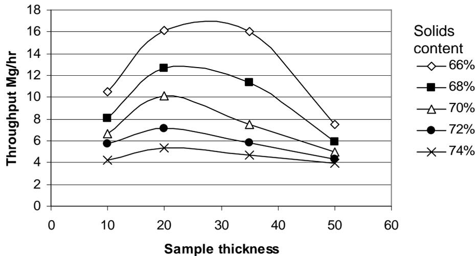
**Figure 5** Optimised throughputs to achieve different target solids contents using 7.5 mm pitch belts
