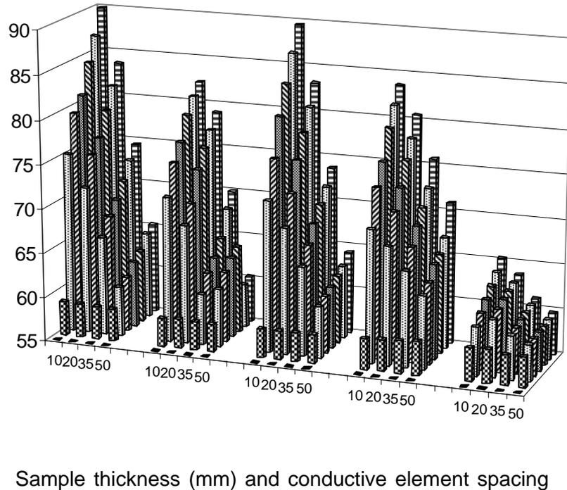
**Figure 4** Dewatering performance of kimberlite slimes from source A at 15 V using all the filter electrodes and control (0V) at 10 mm, 20 mm, 35 mm and 50 mm sample thicknesses
